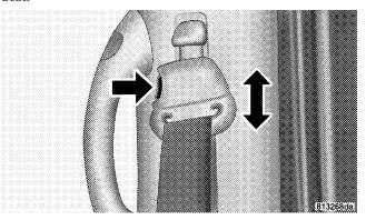
As a guide, if you are shorter than average, you will prefer a lower position, and if you are taller than average, you'll prefer a higher position. When you release the anchorage, try to move it up or down to make sure that it is locked in the desired position.
